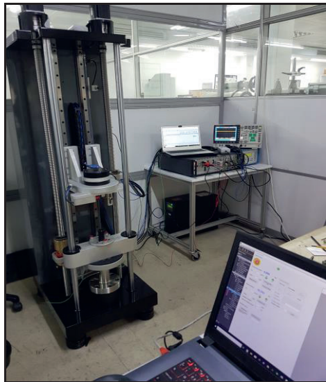
Fig. 2. Dropping mass dynamic calibration system
