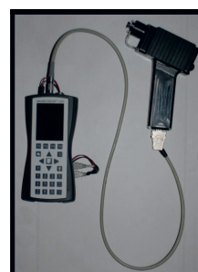
Fig. 1. Handheld prototype (20 x 10 cm) for simultaneous detection of explosives in gas-phase.
