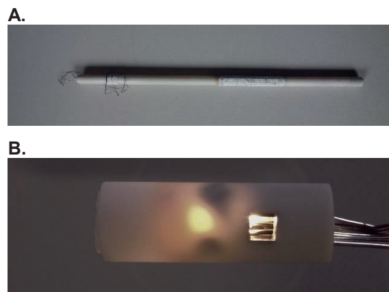
Fig. 3. A. Overview of the YSZ tube with electrodes. B. Part of the ceramic tube with inside illumination at the electrode position. Blackening inside the tube is visible.
