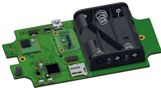
Fig. 3. First functional model in 3D overview with the electronic components of the sensor node.
