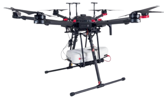
Figure 3: Commercial drone equipped with the methane spectrometer.
