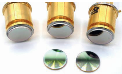
Fig. 2. Photograph of the used sources. From left to right: emitter with parabolic reflector, emitter with Fresnel lens for 4.3 \mu\text{m} (F1) and with Fresnel lens for 10.5 \mu\text{m} (F2).
